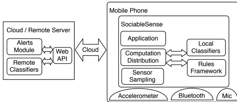
Fig. 3. SociableSense architecture: the data processing and inference tasks are distributed across mobile devices and a cloud-based back-end.
