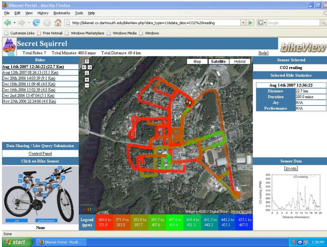
**Figure 4. The BikeView portal provides personal access to archived cycling data, which can be socially shared with cyclists, or used to support a public sensing initiative. The CO<sub>2</sub> map shown here is the result of multiple users' data merged to form a complete map of Hanover, NH, USA.**
