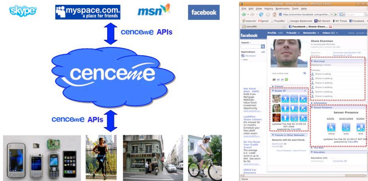
(a) CenceMe distills a user’s “sensing presence” from samples taken from sensors embedded in personal mobile devices (e.g., mobile phone, PDA, mp3 player), sports equipment (e.g., running shoes, bicycle), and the civic infrastructure. Sensing presence is sharable with a user’s friends through popular social networking applications.
