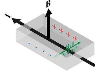
**Figure 1: Measuring the Magnetic Field from a MEMS device. The flow of current ( $I$ ) through a conductor polarizes the material. The resulting voltage between opposite sides is known as the Hall Voltage, from which you can derive the magnetic induction  $B$ .**
