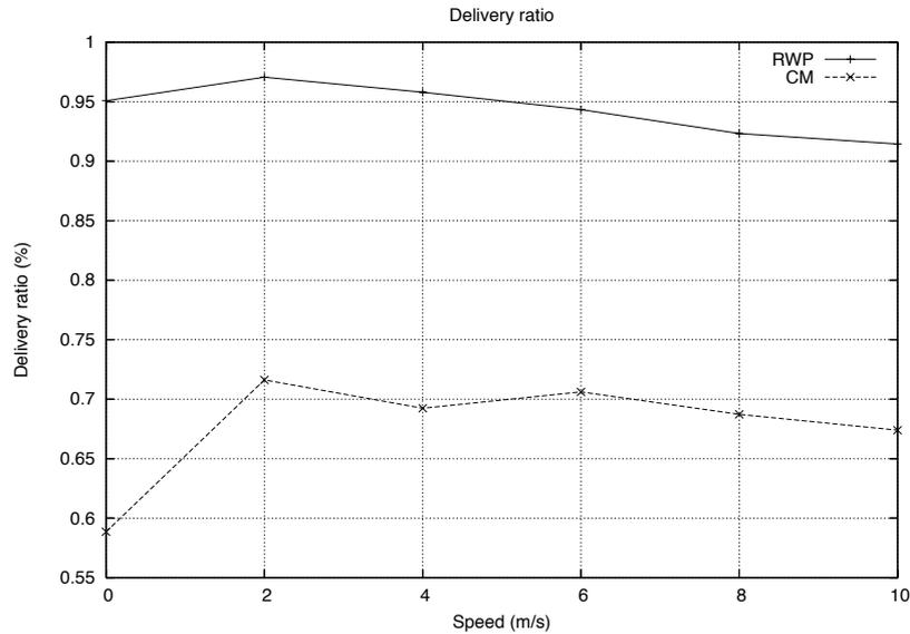
Figure 3.19: Influence of the mobility model on the AODV protocol performance (delivery ratio vs speed).
