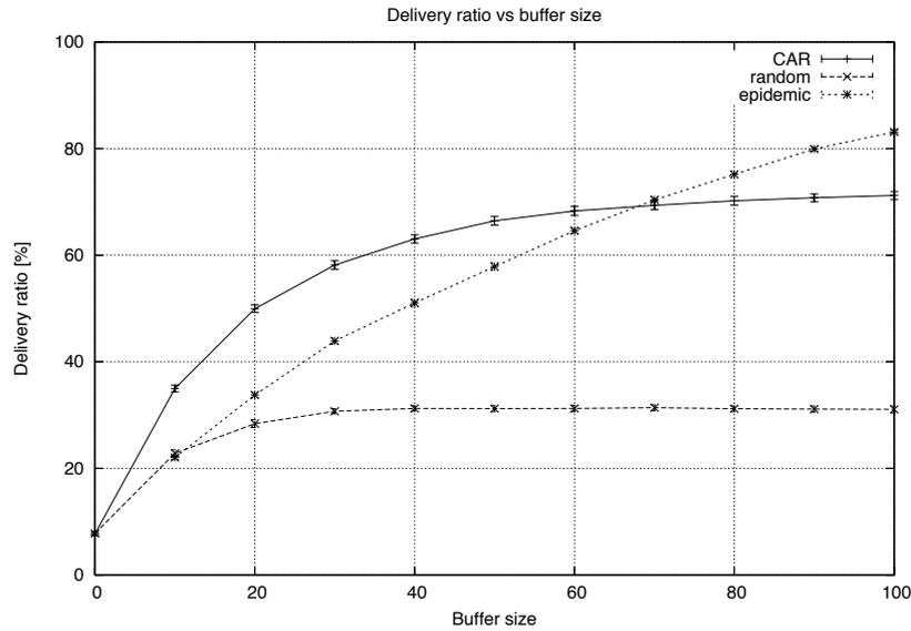
Figure 4.7: Delivery ratio vs buffer size – analysis with very small buffer (scenario with 100 hosts and Community based mobility model).
