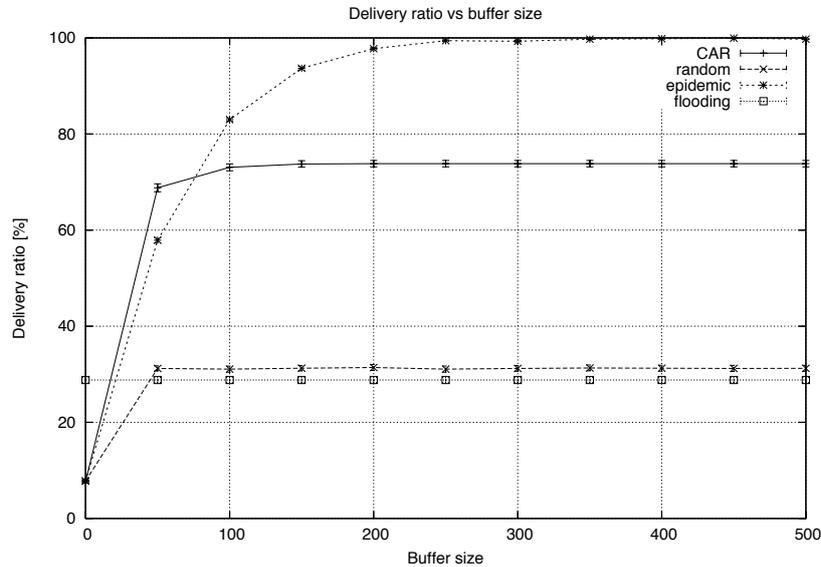
Figure 4.6: Delivery ratio vs buffer size (scenario with 100 hosts and Community based mobility model).
