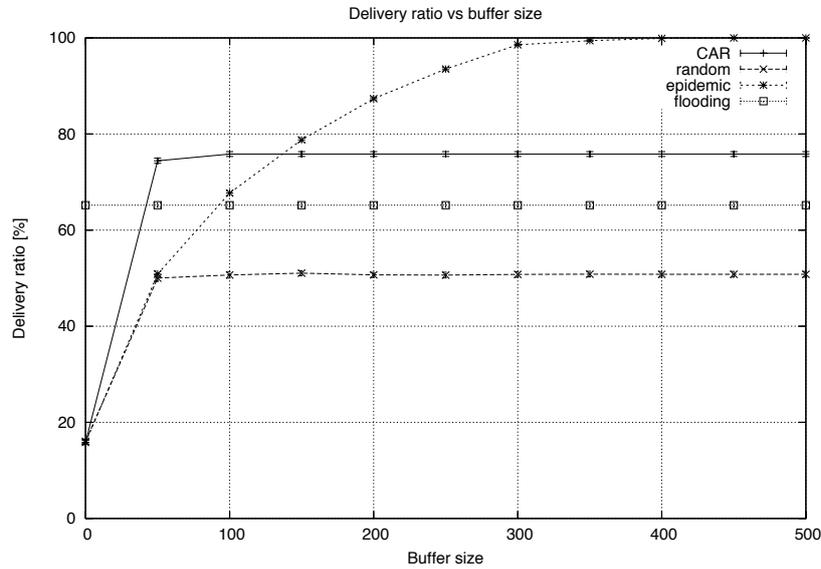
Figure 4.9: Delivery ratio vs buffer size (scenario with 50 hosts and Random Way-Point model).
