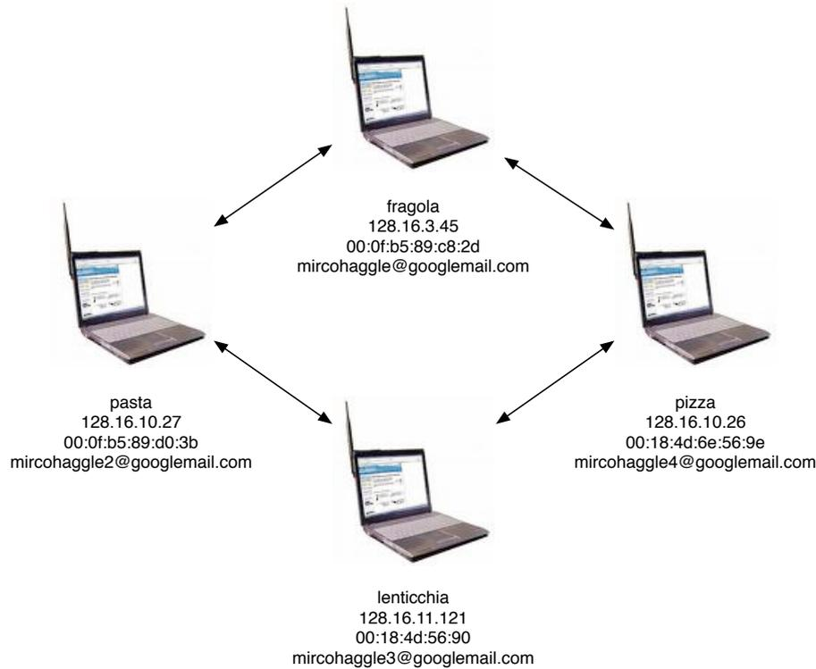
Figure 5.4: Topology and addresses of the hosts of the Haggles testbed.
