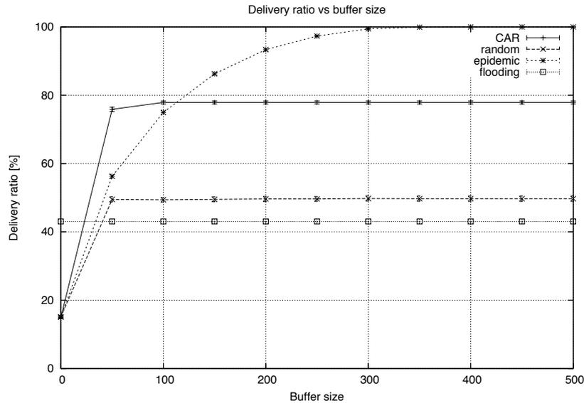
Figure 4.3: Delivery ratio vs buffer size (scenario with 50 hosts and Community based mobility model).
