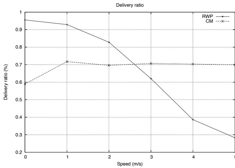
Figure 3.20: Influence of the mobility model on the DSR protocol performance (delivery ratio vs speed).
